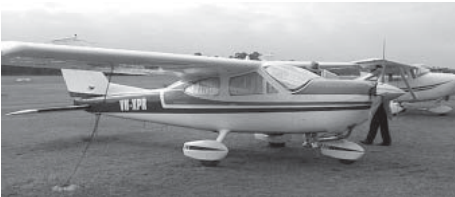
VH-XPR, owned by Ian Poyritt, the only three-blade prop equipped Cardinal at the Hoxton fly-in, also equipped with PowerFlow low restriction exhaust system.
