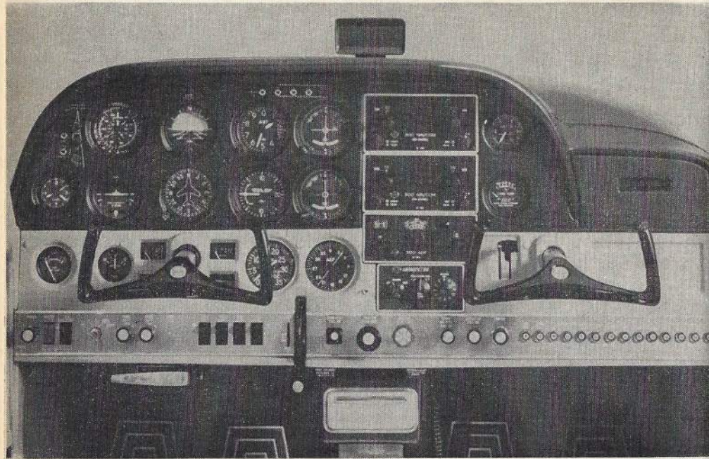
The Cardinal's panel is all new, and is in keeping with the styling of the aircraft. The elevator trim control is at the bottom of the panel, SE of the pilot's control wheel. Note that right side of panel is lowered.
