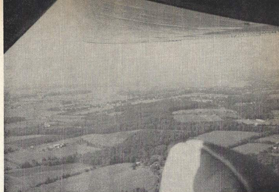
Look, no strut! In this picture it's also possible to see how much twist there is in a Cardinal wing. With the angle-of-attack so much lower at the tip, the ailerons tend to stay responsive at low speeds.
