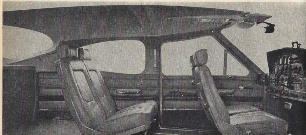
The Cardinal's interior, shown above, is very spacious. It's well finished, too, with a wide choice of materials. An optional child's seat can be installed in the baggage area which has a 120 lb. structural capacity.
